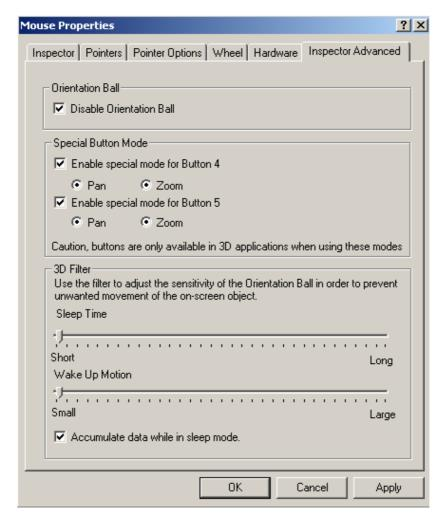
The Inspector Advanced Property Page tab contains options for specialized configuration of the orientation ball and the side buttons.
